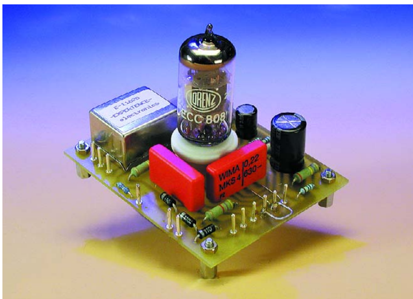
Figure 8. Circuit board layout for ECC808 (board available from Experience Electronics).
